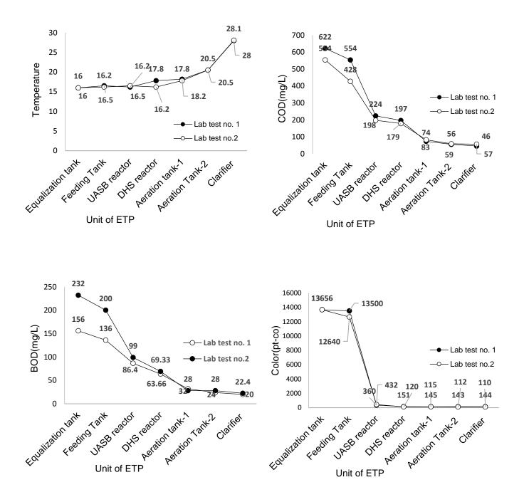
Figure 3: Dissolved oxygenFigyu, pH, turbidity, electric conductivity, temperature, chemical oxygen demand, biological oxygen demand and color profile of UASB combined with DHS treatment process for two laboratory test.
