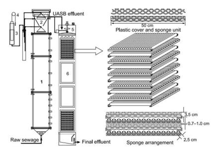
Figure 1: UASB bioreactor combined with DHS reactor
