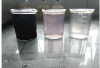
Figure 6: Color variation of wastewater sample of equalization tank, UASB reactor and DHS ŀ reactor.
