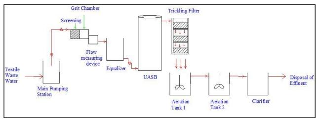
Figure 2: Schematic diagram of the ETP.
